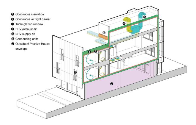
The Passive House is a consequent further development of the low energy house. We reduced the unnecessary heat losses through walls, roofs and windows to the extent that a heating system became completely irrelevant.
