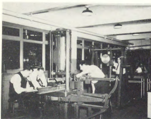
The first class in Materials Inspection and Testing breaking a wood beam and observing deflections and load.
