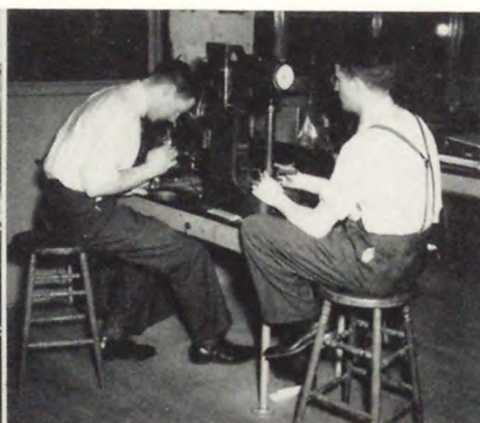
Examination of metal specimens by microscope and Rockwell Hardness Tester in the Metallurgical Laboratory, Newark College of Engineering, in Materials Inspection and Testing Course.
