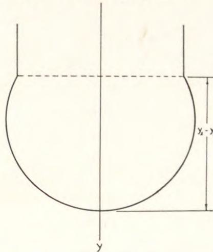
Figure 4. Curve assumed by a rectangular filter cloth
