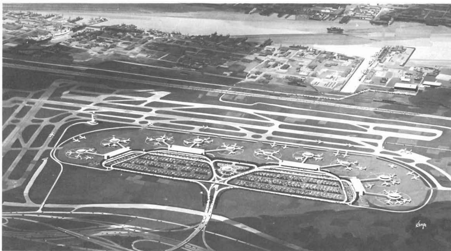
Artist's drawing showing design concept of $125,000,000 redevelopment of Newark Airport now under way for completion in 1971. The program includes 340-acre passenger terminal area with four terminal buildings, parking areas
