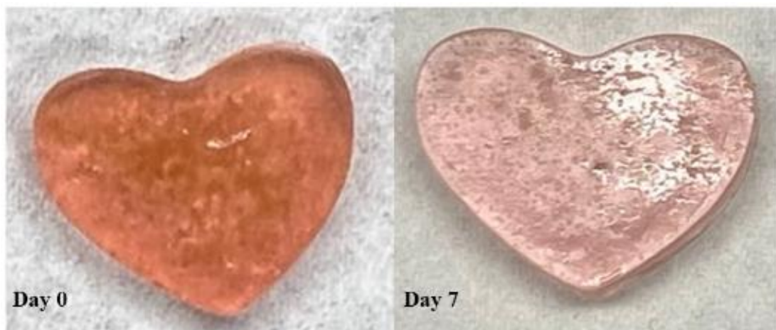
Figure 3.9 Films preparation steps include mixing the PETMP, TMPTMA and BD-I-TMG (ratio: 1 mmol : 1 mmol : 0.05 mmol) in a glass vial, loading the mixtures in the mold, then the mixture was irradiated by the Thorlab's M505L3 LED light source (nominal wavelength 505 nm, power density is 80 mW/cm 2 , irradiated distance: 1 cm) for 30 min. After solidifying, the film was soaked in DMSO for 7 days.
