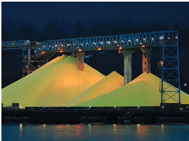
Figure 1.3 Elemental sulfur piles from Claus process.
