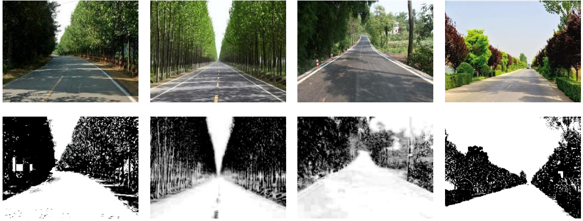
Figure 5.14 Examples of the proposed shadow feature extractor. First row contains some sample road images and the second row represents the corresponding results of the shadow weakening method.
