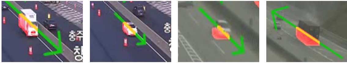
Figure 5.1 Sampling the road pixels from the background image based on the direction of moving vehicles in order to avoid sampling non-road pixels. The red color indicated the location of the sampled road pixels.
