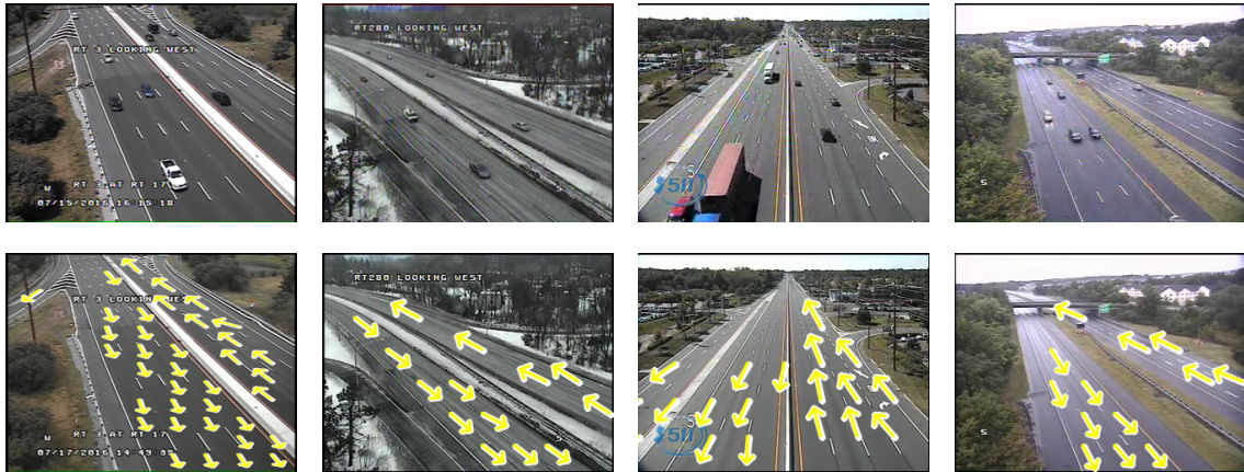
Figure 5.11 Extracting a matrix of motion flow vectors using GMM method with optical flow vectors as input. First row contains sample frames of traffic videos. Second row represents the corresponding flow model matrix obtained from the GMM method.
