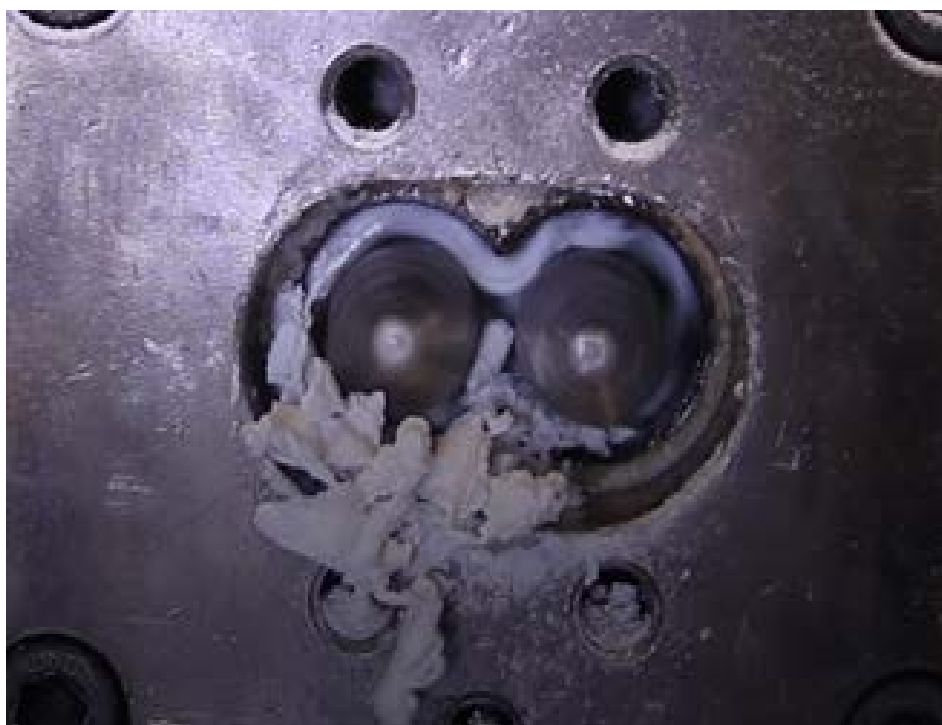
Figure 4.67 Granules for theophylline (THF) and hydroxypropylcellulose EXF (HPC EXF) blend (THF:HPC EXF) at 8 kg/hr.; 200rpm; 50°C.
