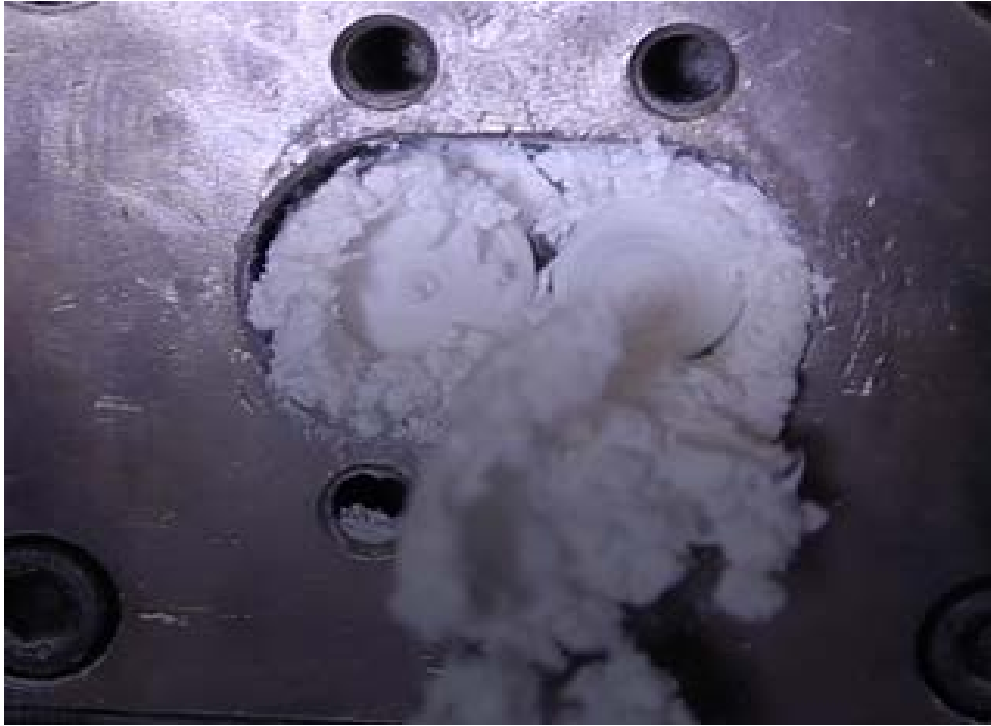
Figure 4.48 Granules and particle size distribution for micronized theophylline (MTHF) and hydroxypropylcellulose MF (HPC MF) blend (MTHF:HPC MF) at 8 kg/hr.; 200rpm; 50°C.
