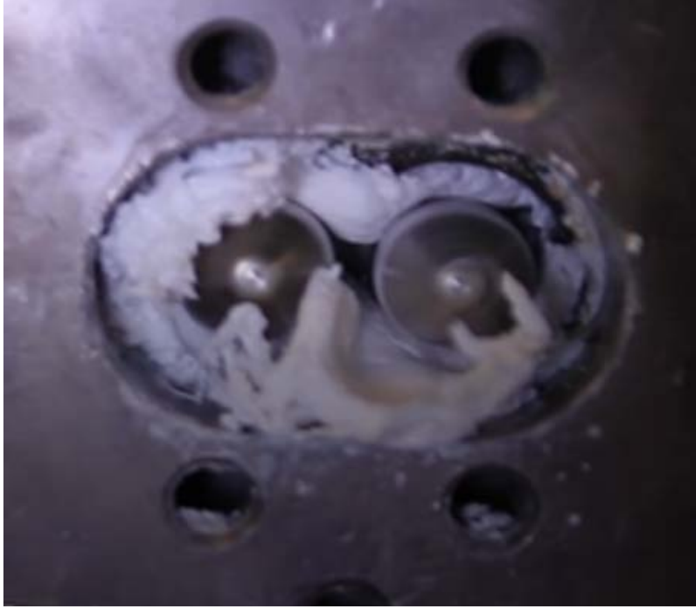
Figure 4.50 Granules for micronized theophylline (MTHF) and hydroxypropylcellulose EXF (HPC EXF) blend (MTHF:HPC EXF) at 4 kg/hr.; 400 rpm; 35°C.
