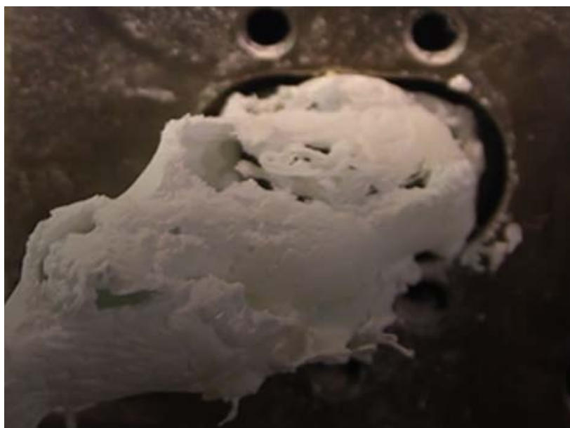
Figure 4.65 Granules for theophylline (THF): hydroxypropylcellulose EXF (HPC EXF) blend (THF:HPC EXF) at 8 kg/hr.; 400rpm; 35°C.
