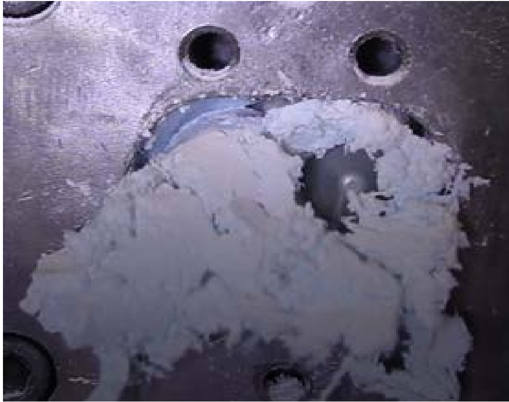
Figure 4.61 Granules for theophylline (THF) and hydroxypropylcellulose MF (HPC MF) blend (THF:HPC MF) at 8 kg/hr.; 200rpm; 50°C.
