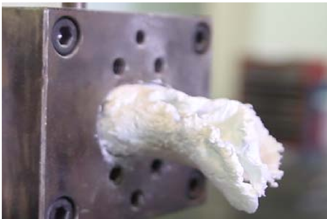
Figure 4.54 Granules for micronized theophylline (MTHF) and hydroxypropylcellulose EXF (HPC EXF) blend (MTHF:HPC EXF) at 4 kg/hr.; 400 rpm; 50°C.
