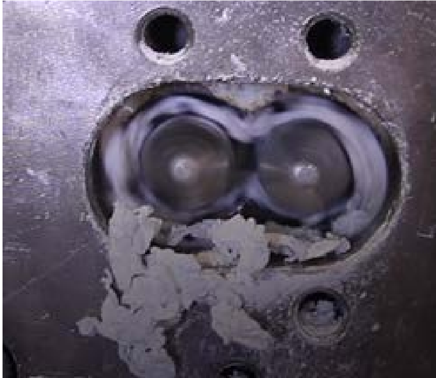
Figure 4.66 Granules for theophylline (THF) and hydroxypropylcellulose EXF (HPC EXF) blend (THF:HPC EXF) at 4 kg/hr.; 200rpm; 50°C.
