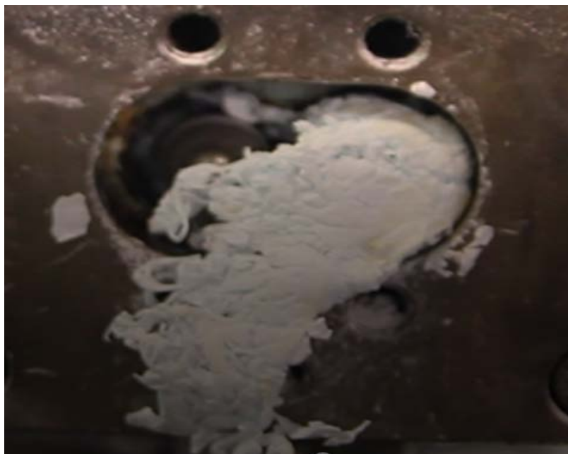
Figure 4.64 Granules for theophylline (THF): hydroxypropylcellulose EXF (HPC EXF) blend (THF:HPC EXF) at 4 kg/hr.; 400rpm; 35°C.
