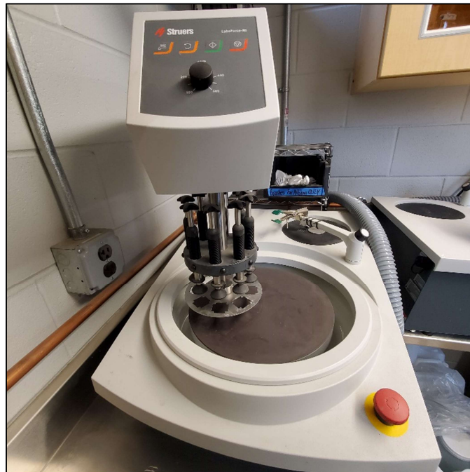
Figure 2.7 LaboPol-30 with LaboForce-Mi counter-rotation sample holder.
