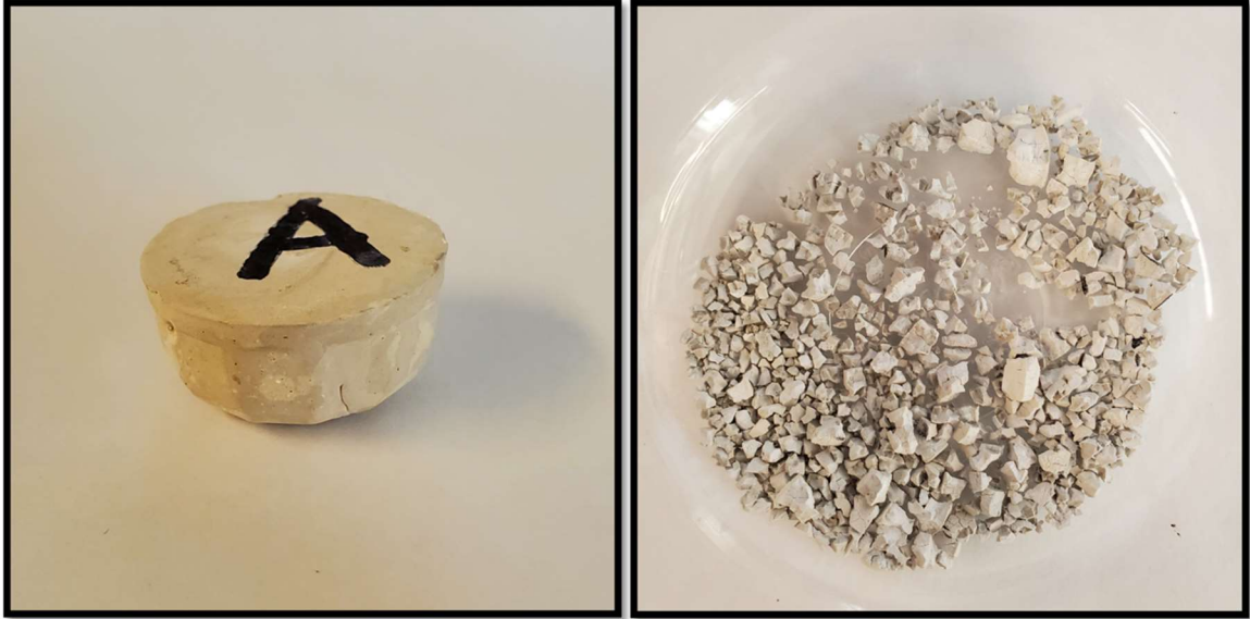
Figure 3.13 Comparison of CSA paste calorimetry specimens in initial state and broken state after seven dehydration and rehydration cycles.
