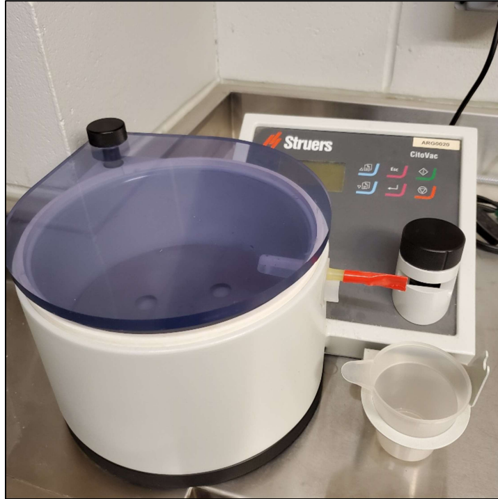
Figure 2.6 CitoVac vacuum impregnation unit.
