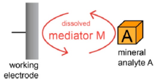
Figure 2.2 Overview of non-mediated (top) and mediated (bottom) electrochemical analyses;
