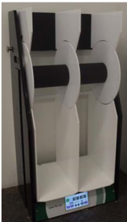
Figure 2.5 Picture of Rotarod apparatus used to assess the motor deficits.
