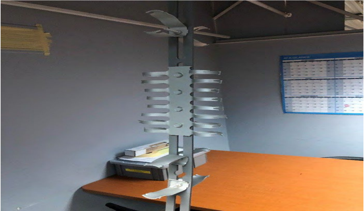
Figure 2.4 Rack used for chemical processing of test specimens in Chapter 3.
