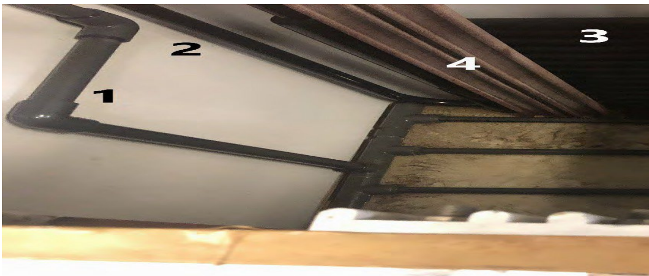
Figure 2.3 (1) Air agitation. (2) Chilling solution. (3) Heating exchanger. (4) Cathode.
