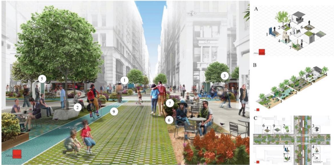
Figure 5.4 Public Square by FXCollaborative. The top image shows a perspective view of a possible street with the fully deployed system of interlocking frames. A: the proposed nine 8'x8' frames. B: A view of four types of themed configuration. From L-R: bike travel and water infrastructure theme, children play area theme, urban agriculture theme, public services (restroom and retail) theme. C: A plan view with the deployed squares, including detailed views of several of the proposed frames.
