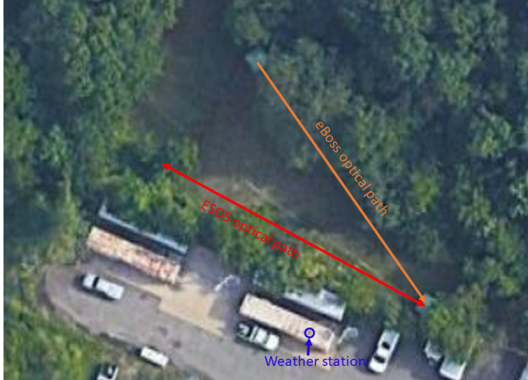
Figure 4.1 Aerial view of the field location ( 40^{\circ}47'09.8''N 74^{\circ}03'28.1''W ). Both green tents, used to protect the equipment from rain, are visible. The optical path of the laser beams, of both eBoss, is indicated by the orange arrow starting from the emitters and pointed toward the receivers. The optical path of the ESOS is indicated by the red double arrow following along the southern tree line. The weather station is located on top of a metal container located directly south of the field and is indicated by a blue circle.
