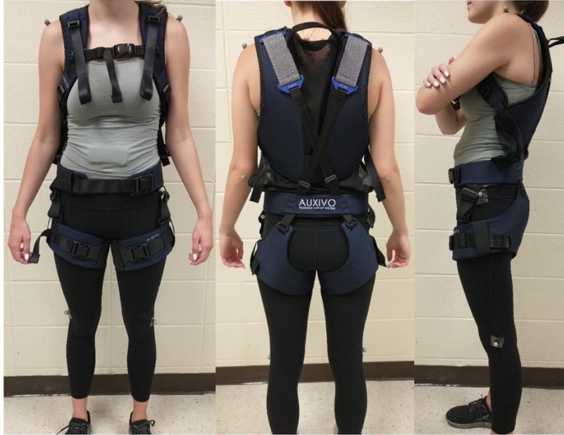
Figure 2.6 A participant wearing the Auxivo LiftSuit (Auxivo AG, Switzerland): front, back and side views. The participant is also wearing the sensors used in the study (e.g., wireless electromyography sensors under shirt, optical tracking markers on shirt, optical tracking markers on shoulders, hips and knees).
