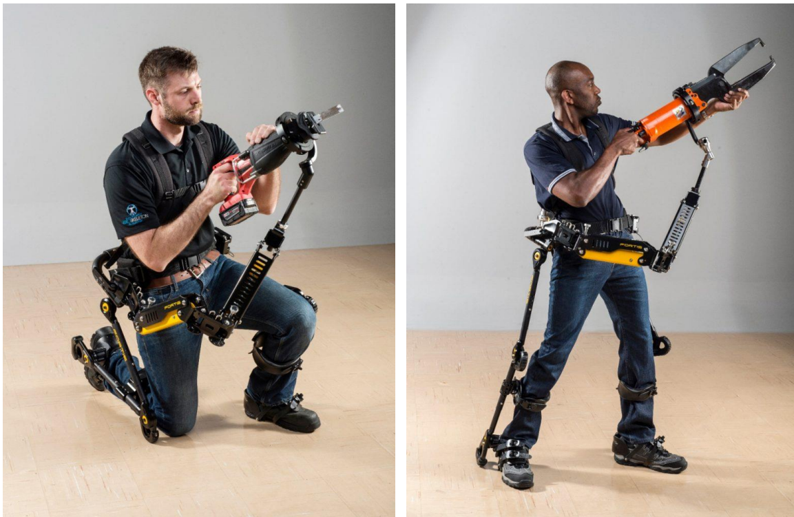
Figure 3.10 Demonstration of Fortis Exoskeleton (Full-Body).
