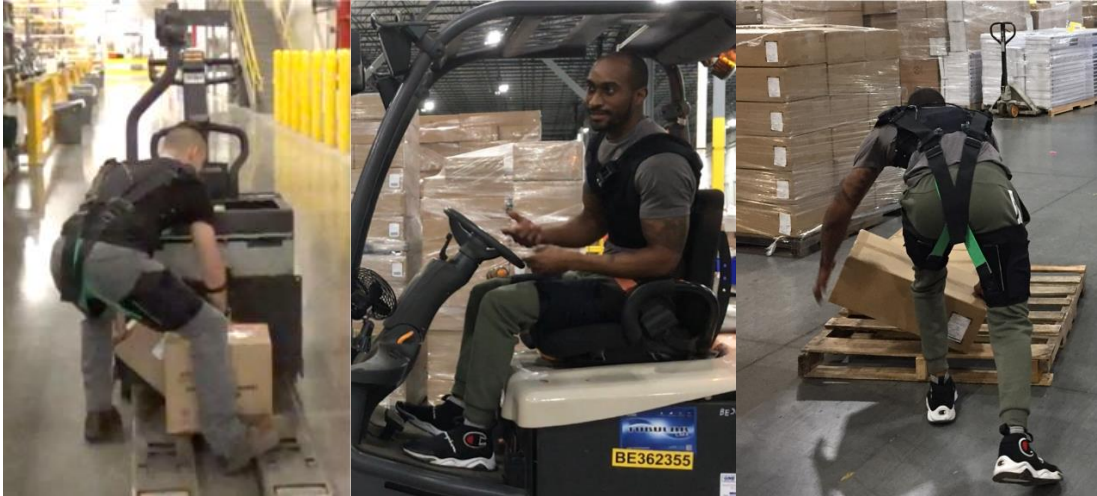
Figure 2.10 Distribution center workers using an exosuit prototype on the job for a variety of logistics tasks: picking, palletizing, forklift driving.
