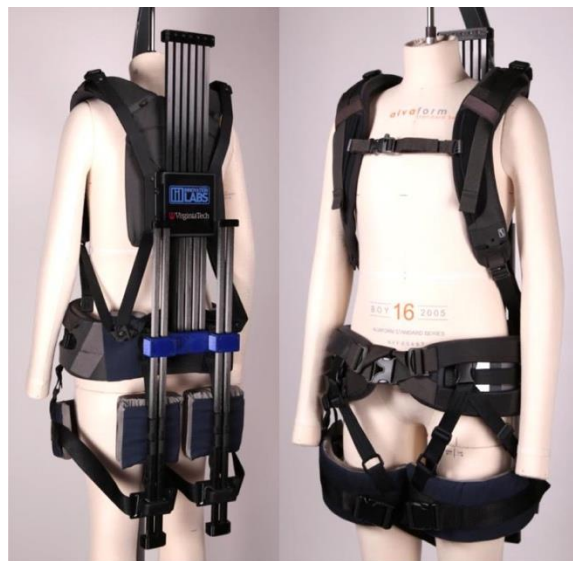
Figure 2.7 Front and back views of the VT-Lowe's exoskeleton.
