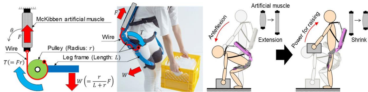
Figure 2.5 Conceptual mechanism for lower back support with the Muscle Suit. (a) Standard model generating active assistive force. (b) Standalone model generating passive assistive force.
