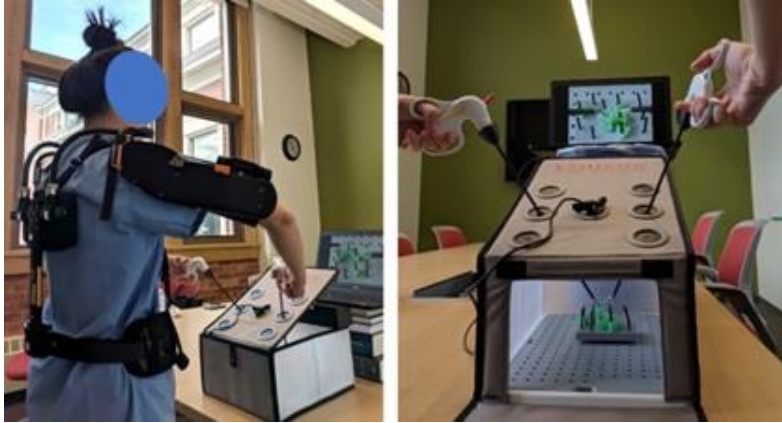
Figure 3.2 Experimental setups for simulated Laparoscopic Surgery task in Cha et al., 2020.
