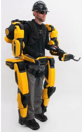
Figure 1.1 Battery-powered full-body exoskeleton - Sarcos Guardian XO Max.
