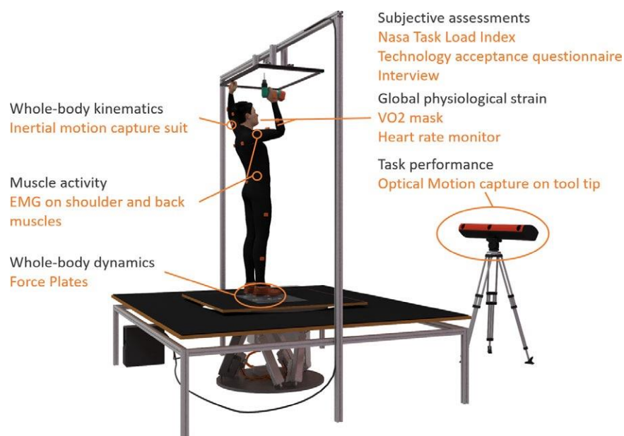
Figure 3.9 Experimental set up for data recording at the laboratory experiment.
