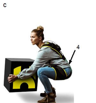
Figure 2.1 Passive back-support exoskeletons mechanical structures and force generation mechanisms.
