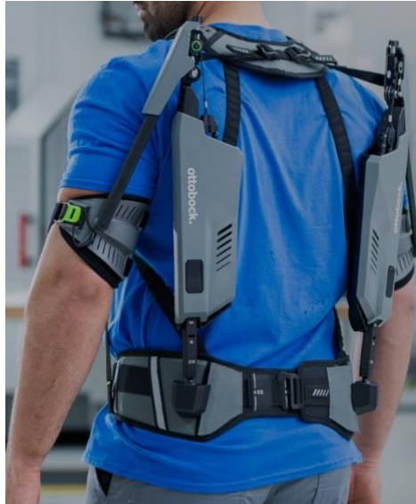
Figure 3.8 Configuration of Paexo Shoulder support exoskeleton.
