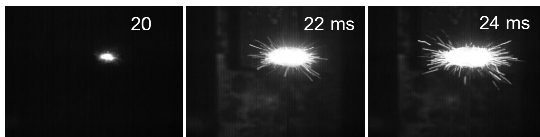
Figure 2.9 A characteristic sequence of video frames showing ignition of S4 (milled in 25% ACN). Heating rate is 34700 \pm 1500 K/s.
