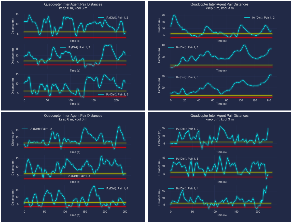
Figure 3.12 Top Row: Inter-sUAV distances for 3 quadrotors (Top Left: HWIL and Top Right: Field Test) Bottom Row: Inter-sUAV distances for 3 pairs in the 4 quadrotors test (Bottom Left: HWIL and Bottom Right: Field Test). Both results demonstrate that the flocking controller maintained the required separation k_{sep} and collision avoidance k_{col} distances for most of the test duration. Any minor breaches of the k_{col} were corrected quickly and safely.
