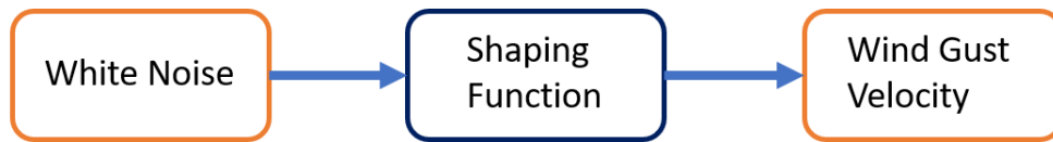
Figure 2.14 Filtering process for Dryden and von Kármán wind generation models.
