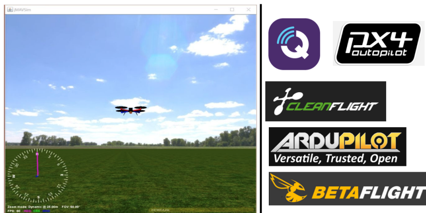
Figure 6.4 (Left) Snapshot of JMAVSIM flight simulator for the quadrotor. (Right) SITL software tools Qground control, and PX4 autopilot.
