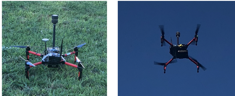
Figure 2.7 FT-205 wind sensor mounted on the DJI Matrice 100 sUAV to collect wind data during flight test.
