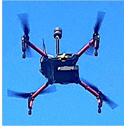
Figure 3.10 FT-205 wind sensor mounted on the DJI Matrice 100 sUAV to collect wind data during flight test.
