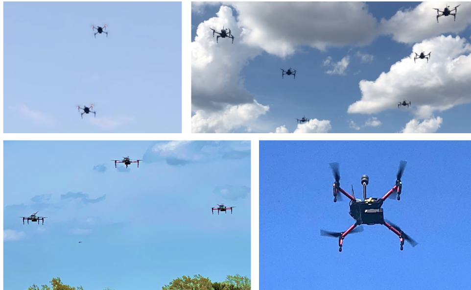
Figure 4.1 Snapshots of a 2 quadrotors (top row left), 3 quadrotors (bottom row left), 6 quadrotors (top row right) operating outdoors. Bottom row right image shows the FT-205 wind sensor mounted on the DJI Matrice 100 quadrotor to collect wind data during flight test.
