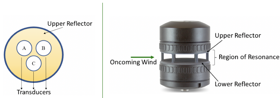
Figure 2.6 Left Image: Alignment of transducers on the upper reflector for an acoustic resonance ultrasonic anemometer. Right Image: Side view of the FT205 acoustic resonance ultrasonic anemometer.
