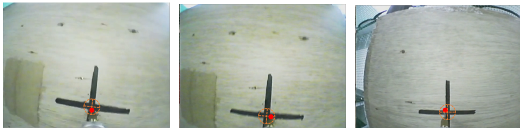
Figure 5.9 The drilling accuracy over all the three aerial drilling tests.
