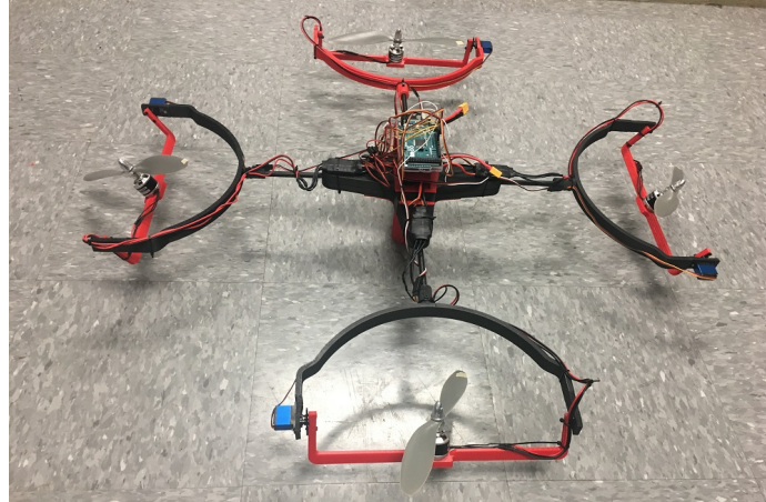
Figure 2.5 A prototype of the proposed dual-axis tilting vector thrust UAV.
