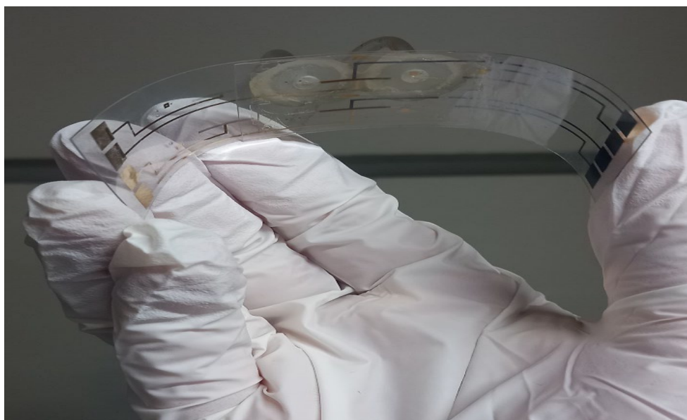
Figure 3.4. Flexible Non-Planer Interdigitated Micro Electrodes Packed with MOF (FNP-ID \mu E).
