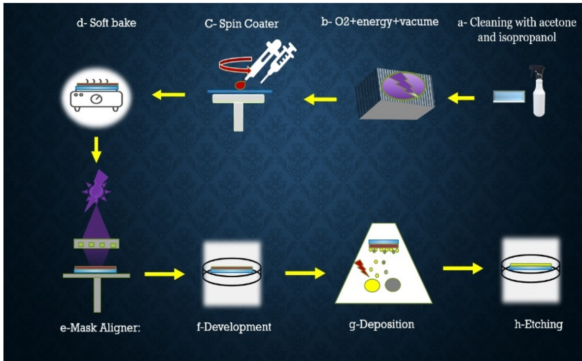
Figure 1.1. Schematic diagram of the lithography process, (a): cleaning, (b) Ozone cleaner, (c): spin Coating application, (d) soft bake, (E): Mask aligner (f): Developing (g): E-beam vapor deposition (h) lift-off process.
