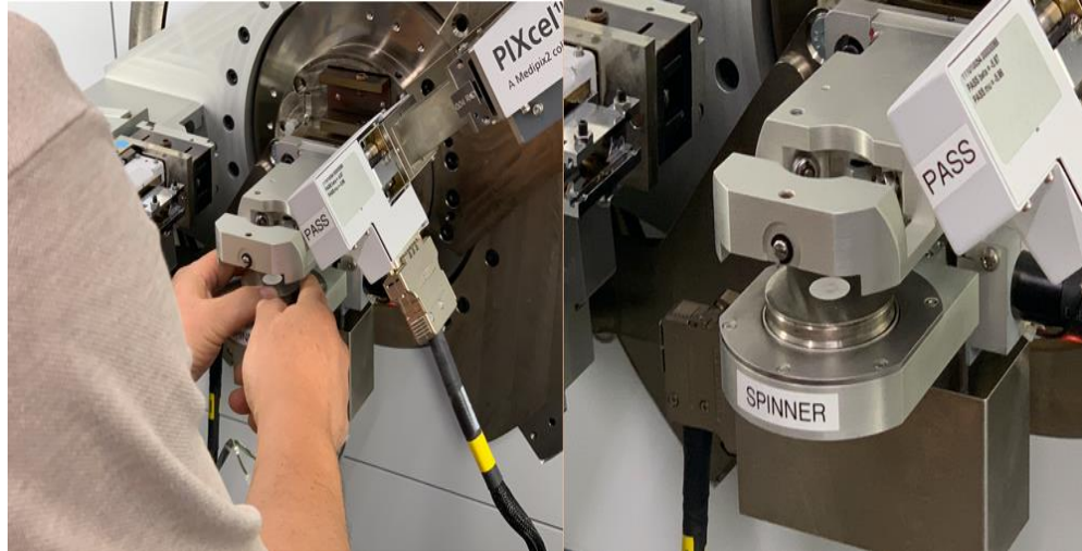
Figure 3.12 Sample mounting. 1) Placing the sample; 2) Sample position and placement.
