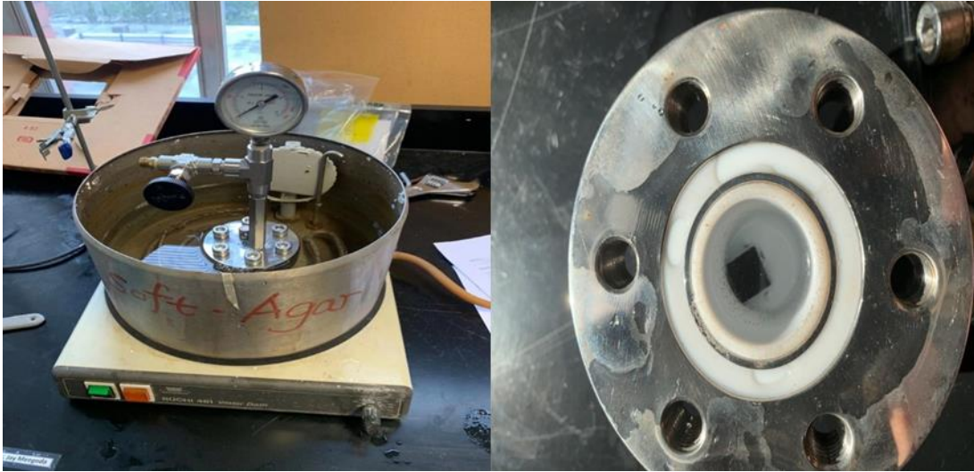
Figure 3.7 Combination of the water bath and hydrothermal reactor.
