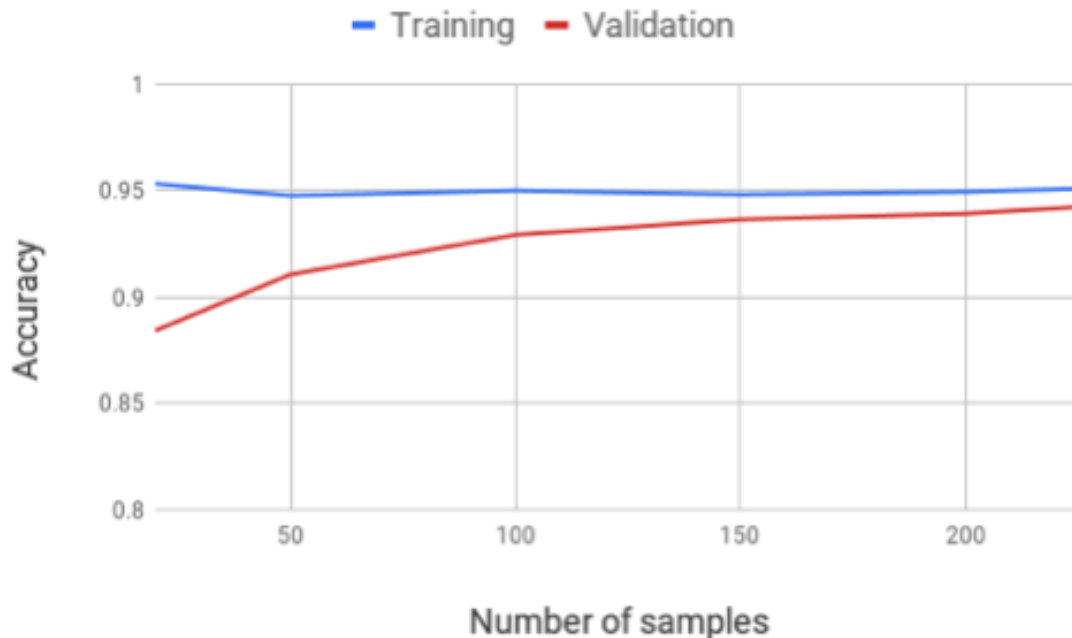
Figure 5.2 Training and validation accuracy of our training and validation folds as a function of sample size.
