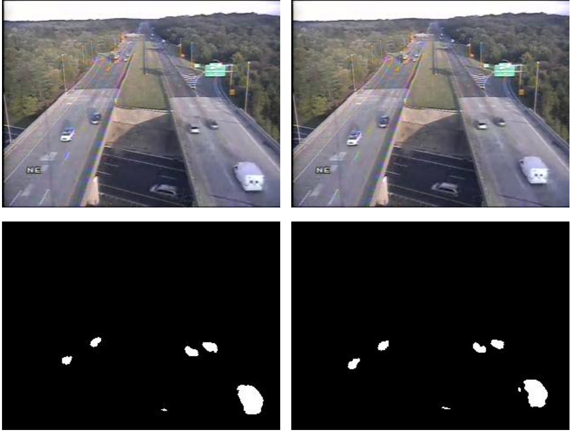
Figure 6.2 Two adjacent video frames from the NJDOT video and their corresponding foreground masks.
