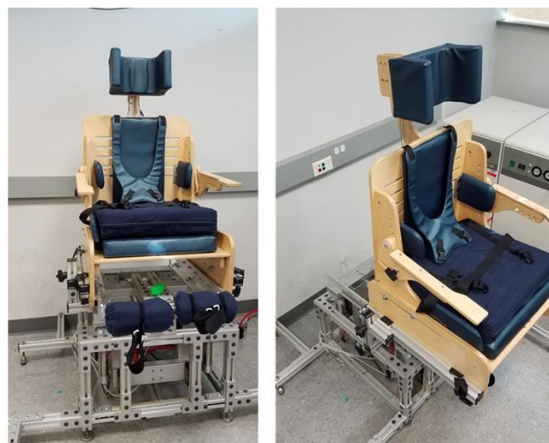
Figure 3.3 Vestibular stimulation chair in the stimulation position (left) and pulled forward for administering the PKD (right).
