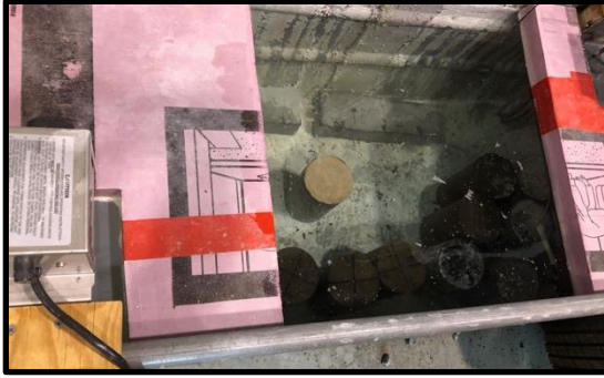
Figure 1.12 Heated curing tank at 50°C (left) and temperature relays set at temperature of 50°C±2°C (right).
