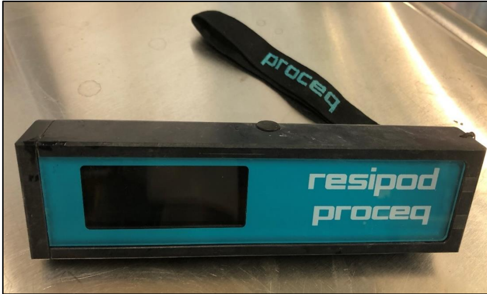
Figure 2.4 The wenner probe for electrical surface resistivity measurement.
