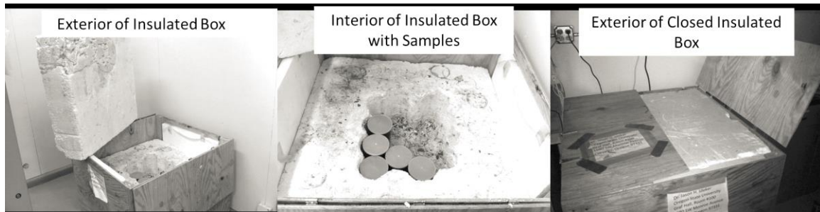
Figure 1.11 Semi-adiabatic insulated box for curing CAC. Source: [88]
