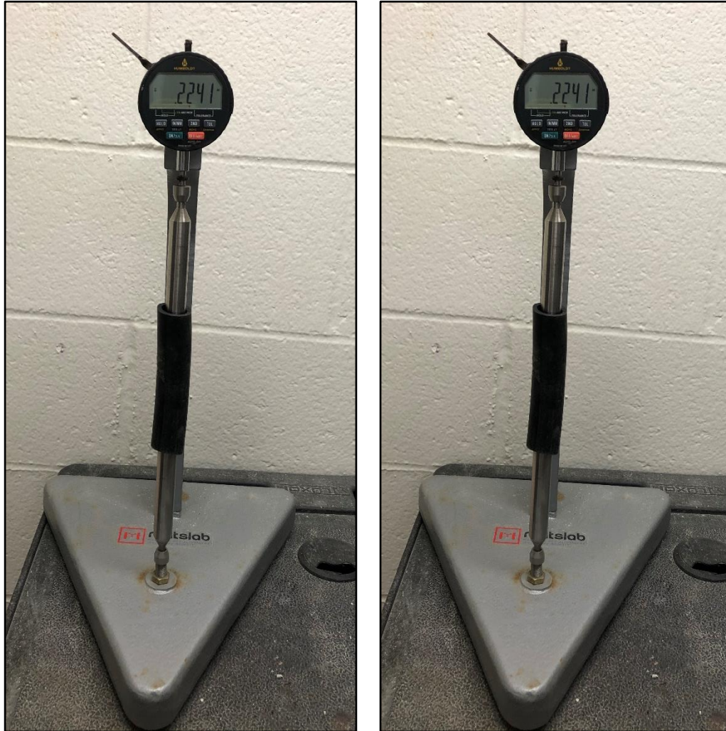
Figure 2.3 Drying shrinkage comparator setup.
