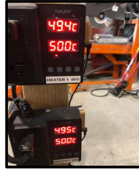
Figure 1.12 Heated curing tank at 50°C (left) and temperature relays set at temperature of 50°C±2°C (right).
