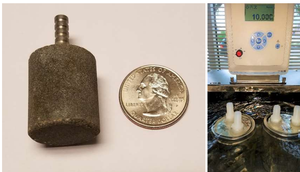
Figure B.1 Diffuser used for ozonation and the constant temperature baths.
