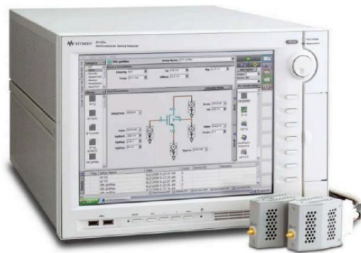
Figure 3.2 Picture of Keysight B1500 semiconductor device parameter analyzer.
