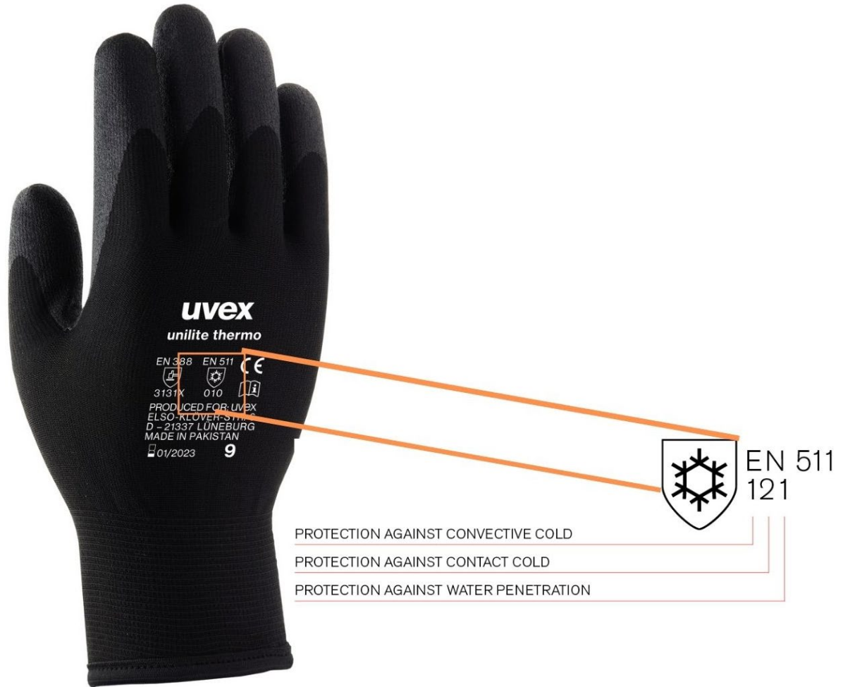
Figure 4.6 Glove manufacturers who have adapted the European Standard EN 511:2006 print the gloves rating on the back hand of the glove.
