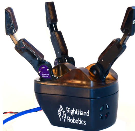
Figure 4.3 ReFlex Takktile hand.
