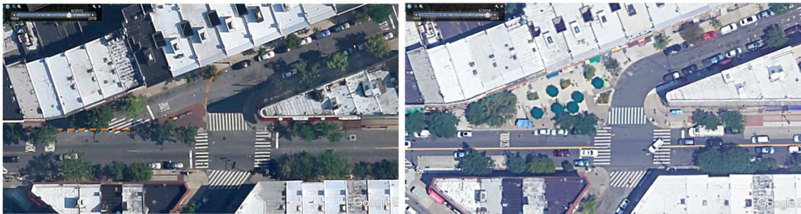
Figure 7.3 Creation of 71 st Avenue Plaza by using residual space between sidewalk and the traffic island.
