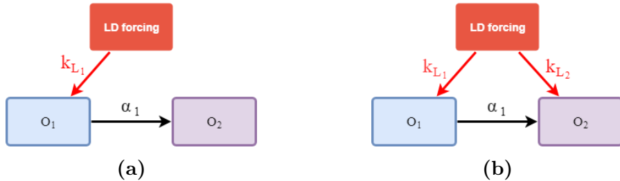
Figure 3.13 (a) Model with strict hierarchical coupling. (b) Semi-hierarchical model when both oscillators receive light input, but the light into O_2 is much weaker than the light into O_1 .
