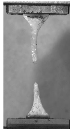
Figure 2.7 Representative image of speckled Type 5 tensile sample, (A) The tensile sample of PSSM ready for test prior to loading (B) The tensile sample of PSSM at failure
