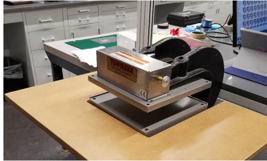
Figure 2.2 Pneumatic die press for cutting samples with standard and custom dies.
