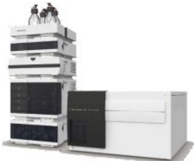
Figure 2.4 Agilent 6470A LC-QQQ instrument.
