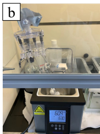
Figure. 2.7 Elution and extraction processes with (a) sample extraction and (b) water and methanol removal.
