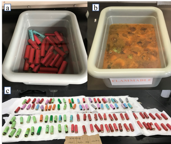
Figure 2.3 Discharge process (a) LIBs in 10 wt. % NaCl solution; (b): after 48 hours discharge; (c) air dried LIBs after washed with DI water.
