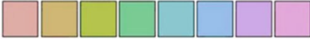
Figure 2.10 Eight color samples employed for calculation of CRI. Source: [141].
