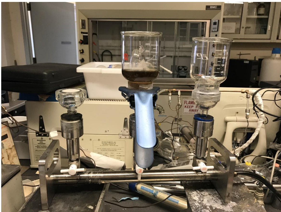
Figure 3.1 The vacuum filtration system used to produce CNTs nanopaper.
