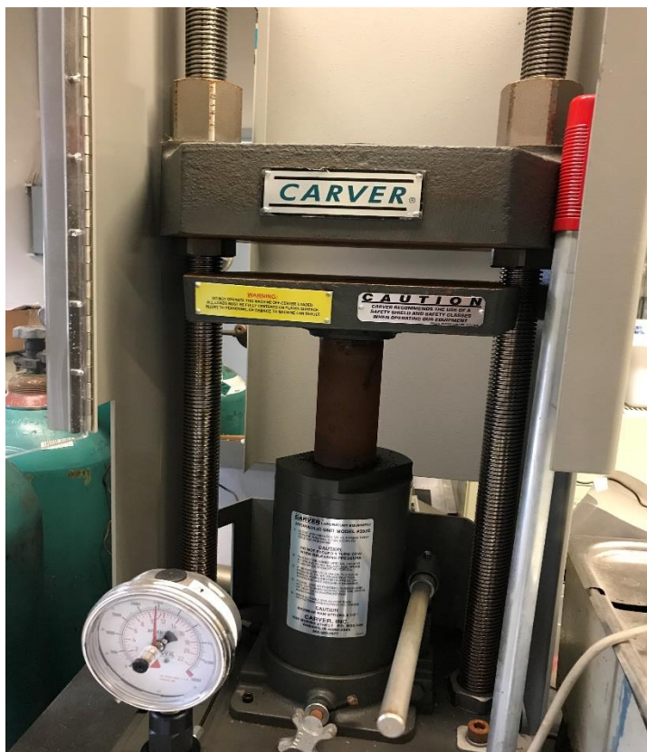
Figure 3.4 The Carver press used for the mechanical compression process.
