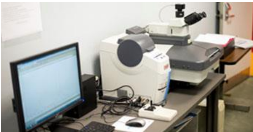
Figure 1.16 Thermo Fisher DXR Raman Microscope used for Raman scattering studies in this dissertation. [55]
