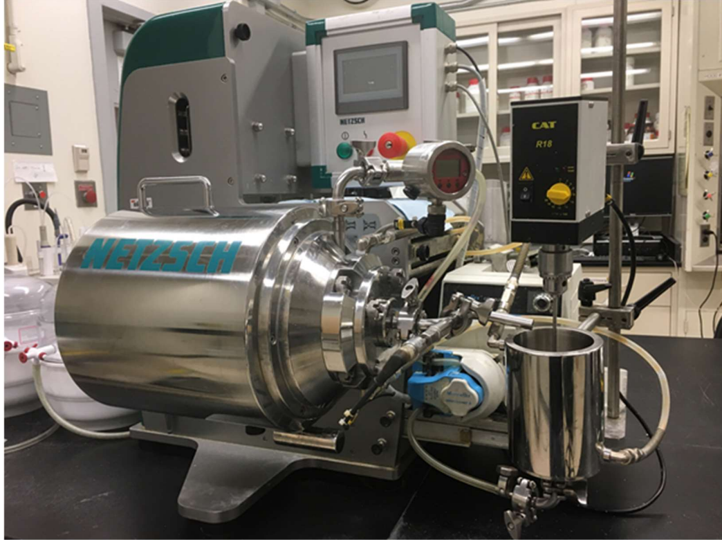
Figure 2.1 Image of the Netsch (Microcer) wet stirred media mill in recirculatory mode.
