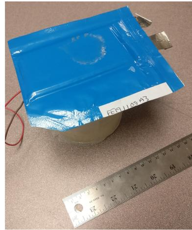
**Figure 3.107** Experimental large battery on coil.
