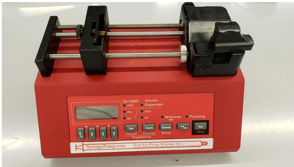
Figure 5.5 NE-1000 Syringe Pump.
