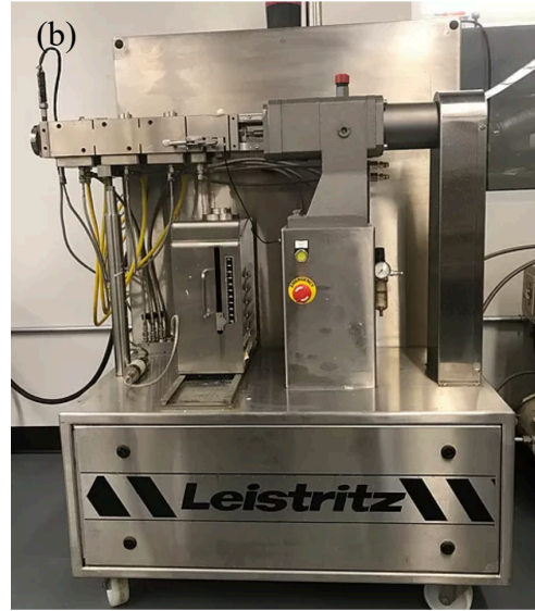
Figure 2.2 Hot melt extruders (a) Single screw extruder from Filabot, (b) Twin screw extruder from Leistritz
