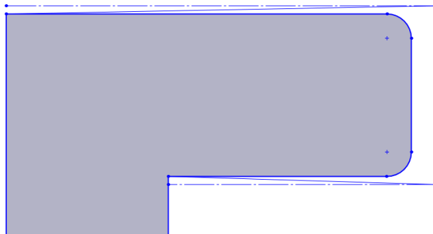
Figure 3.16 Join starting points of the leg with points of intersection between flares and extension for leg length less than 3/8 inches.
