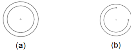
Figure 3.31 (a) Counterbore and Clearance hole pattern, (b) Drill and Tap hole pattern.
