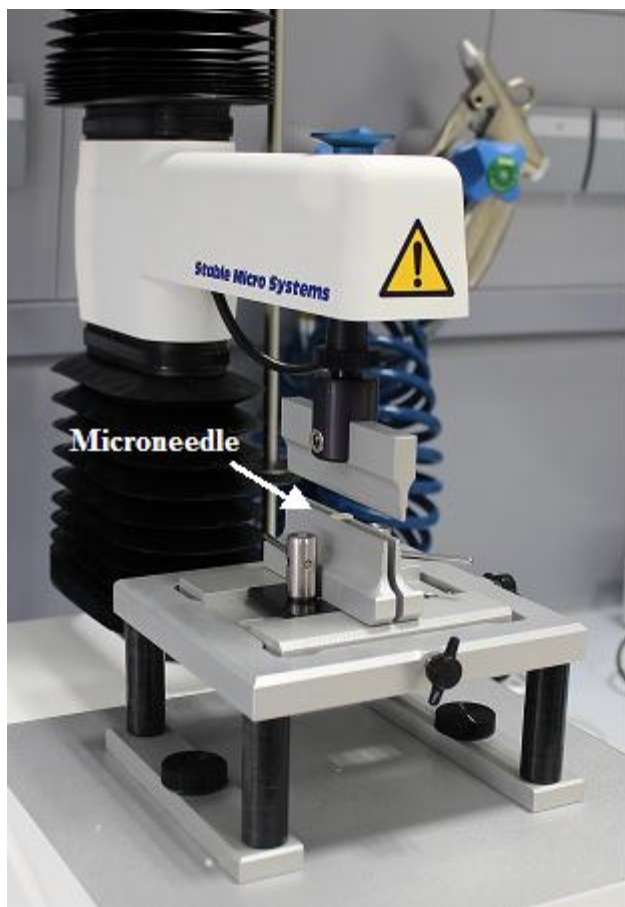
Figure 2.2 Set-up of three-point bend apparatus for testing mechanical strength of microneedle array.
