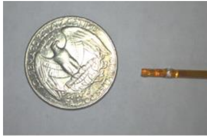
Figure 2.2 qOCE probe compared to a US quarter.
