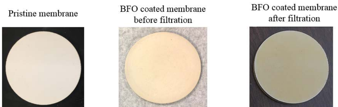
Figure 6.33 The photos of pristine membrane, BFO coated membrane before and after filtration experiments.
