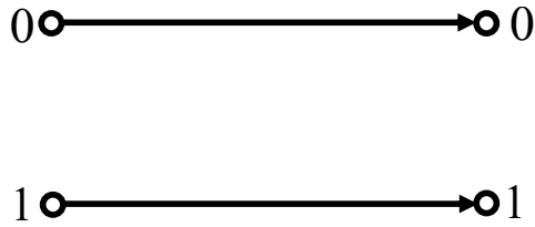
Figure 1.4 Error Probability in a noiseless channel.
