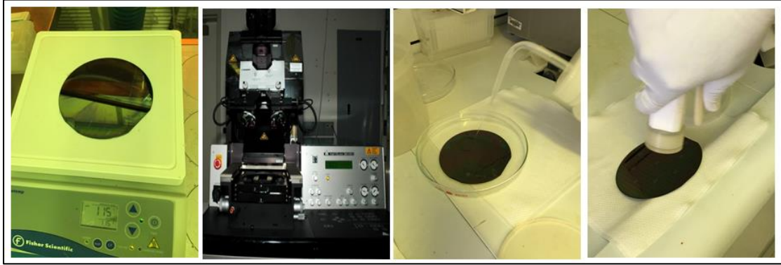
Figure 2.6 Si wafer with photoresist on hot plate, Karl Suss MABA6 mask aligner for UV exposure, developing the Si wafer with CD-26 & Drying Si wafer with nitrogen gun (left to right).
