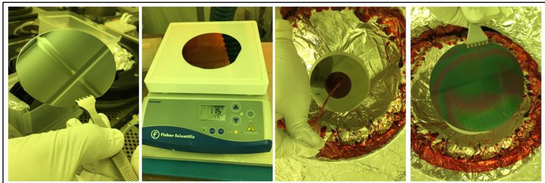
Figure 2.5 Silicon wafer for photo lithography process, Silicon wafer on hot plate, Spin coating the photoresist on Si wafer & Si wafer with photoresist (left to right).
