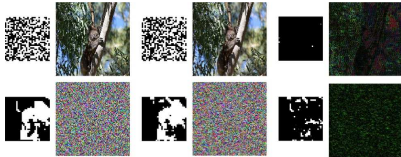
Figure 5.13 Embedding involving noise images. 1st column: the watermark, 2nd column: the cover image, 3rd column: the extracted watermark, 4th column: the marked image, and 5th and 6th columns: the residual errors.
