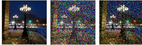
Figure 5.15 Extreme cases. Left: the original marked image. Middle: Gaussian additive noise with variance 20%. Right: 20% Random modificative noise.
