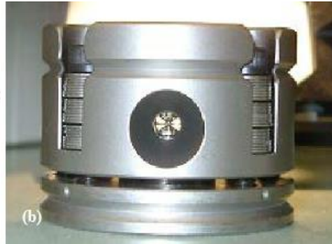
Figure 3.12 (a) Schematic diagram of a DAC (b) the screw-driven DAC used in this work
