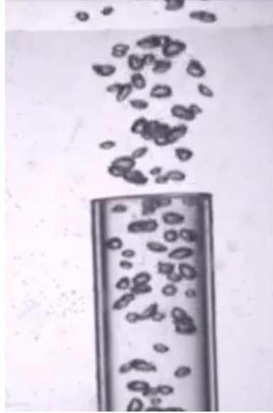
Figure 5.3 Bubbly flow at the near-to-orifice region.
