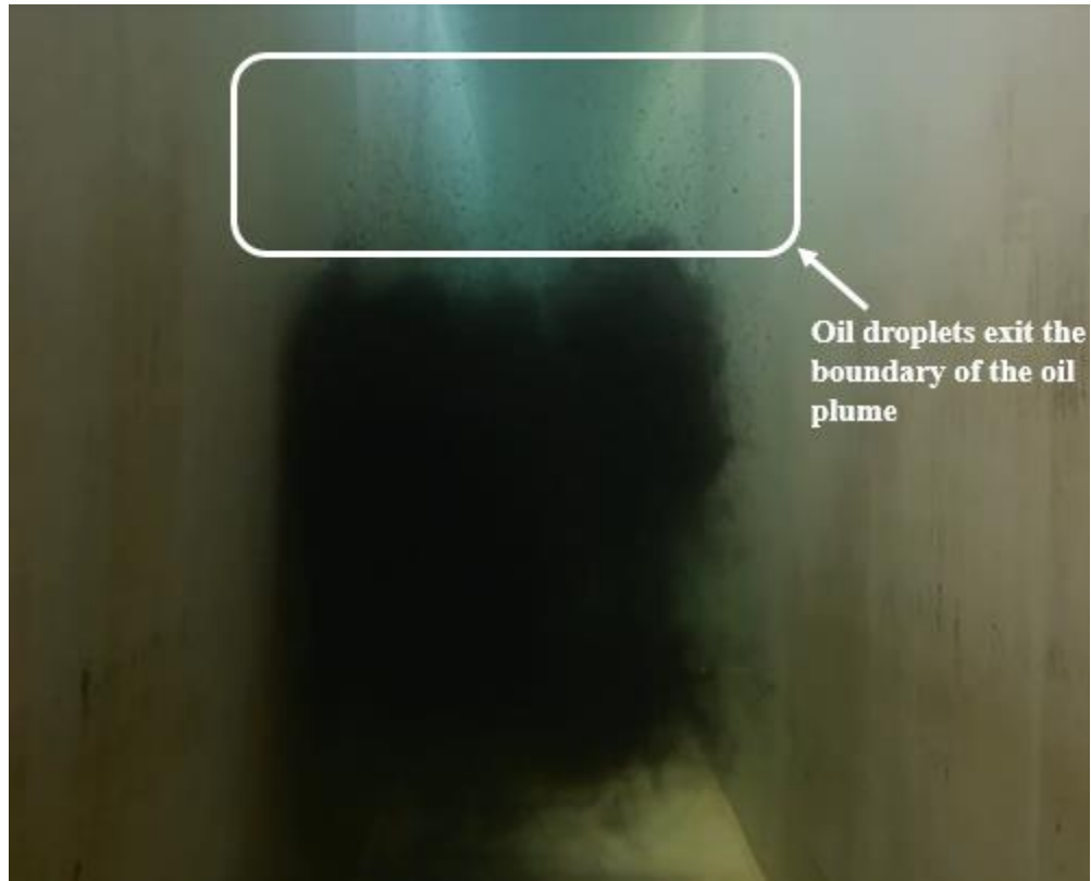
Figure 3.1 Crude oil plume cross-section captured by the high resolution camera at the 4.0 m downstream of the jet orifice. Some oil droplets exit the upper boundary of the plume and continue to rise up (see the details within the white box in the figure).
