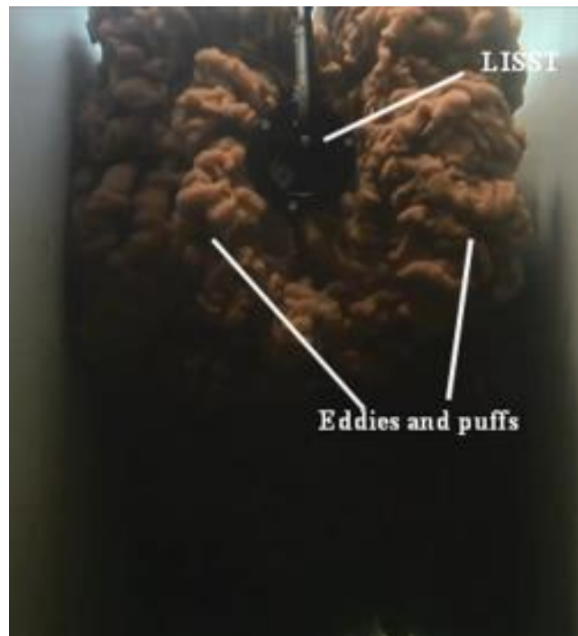
Figure 3.4 Image of oil jet engulfing at the downstream during the experiment (oil with dispersant). Large eddies and puffs were formed and likely increase the mixing of droplets in comparison to that provided by the Reynolds Average Navier Stokes (RANS) simulations.
