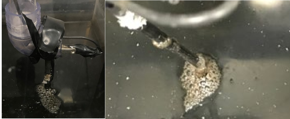
Figure 6.5 Examples of the foam that formed around the electrode on the reservoir surface.
