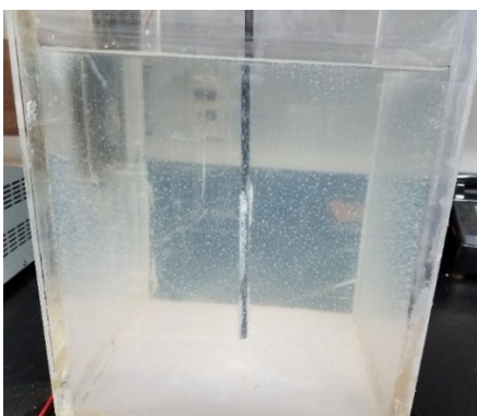
Figure 6.4 Image taken of white precipitate forming on cathode electrode and in its reservoir.
