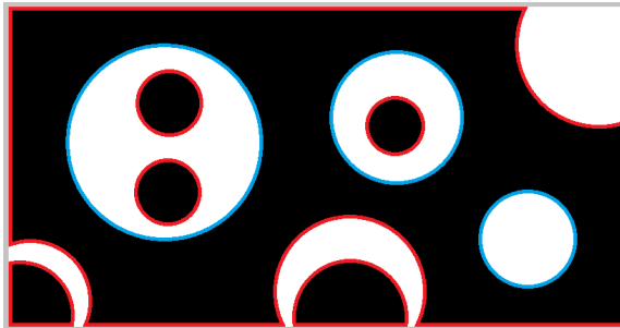
Figure 5.10 The Betti numbers of the above image are b_0 = 3 (white regions with blue outline) and b_1 = 5 (black regions with red outline). Note that white regions, b_0 , that connect with the boundary (gray border) are not counted; however, black regions, b_1 , that connect with the boundary are counted.
